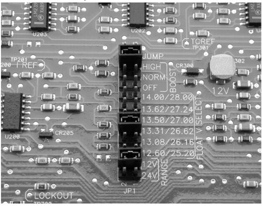
C. For NFPA-20 fire pump applications, set the boost mode jumper (JP1B) to the HIGH setting.
